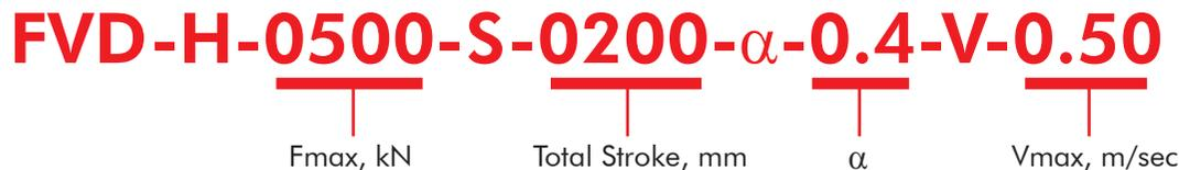
Ordering Example - Stroke=1000mm( $\pm$ 500mm), C=400kN/(m/sec) $^\alpha$ ,  $\alpha$ =2.0, Vmax=0.7m/sec
